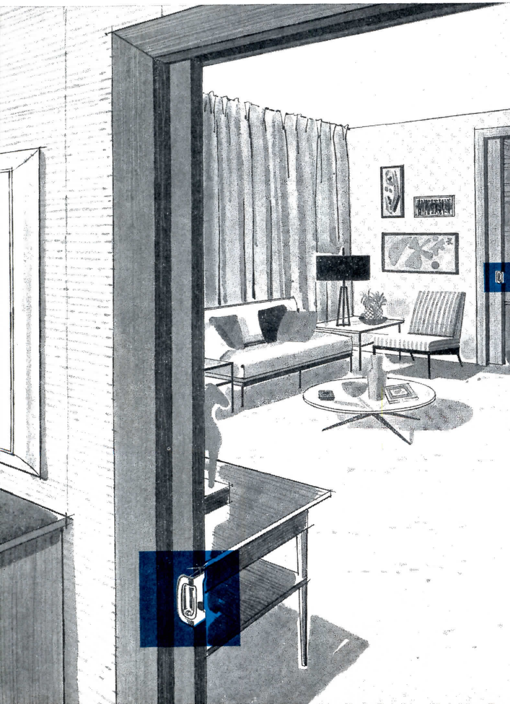
Pocket Door Lock For bathroom and bedroom doors where privacy is desired. Simple installation with standard boring jig.
