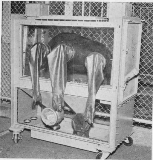
Biological research labs have been built on both "DDD" and "CC" concepts of lab use. Animal housing facilities are sometimes provided in lab building proper, sometimes in separate pens as at Hanford (right). Box labs of special design (left) provide completely controlled environment and mobility of unit for more flexible use of space; care of animal and experiment conditions are simplified
