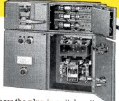
Notice how the plug-in switch unit is mounted directly above the starter, permitting interlocking. The starter cannot be opened when the switch is in the "ON" position.
