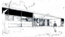
Glass at top of Smithtown window wall is dark enough to control glare, luminous enough to minimize contrast with lighter gray strip below. Lowest section is almost-clear gray glass
