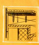
Typical detail and photo of Kaiser Aluminum's Type K-1 Gravel Stop. Note simplicity and pleasing shadow line that results from the straight drip edge feature.
