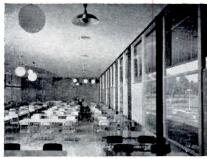
At John Jay High School, Cross River, N.Y., a strip of glare-reducing glass is dropped from the overhang to control sky glare on the cafeteria window wall. The semi-recessed downlights that form the base for the interior lighting are accented by low-hanging clusters of vari-sized incandescent globes
