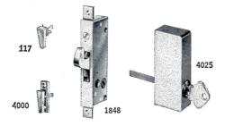
The 1848 Sliding Wall Deadlock shown above measures only  $3\%'' \times 11/8'' \times 1/2''$ , has a collapsible bolt for protection of door and lock, and operates with positive "feel appeal". To compensate for possible misalignment of door and jamb, bolt projection can be adjusted a full %'' by simply turning a screw in the lock face. The 4025 cylinder group is a clean-lined outside pull, offering key control that can be keyed-in with most popular cylinder systems.
