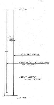
Details of representative vertical luminous elements resemble those for luminous ceilings. Lamps are shown mounted both vertically and horizontally within the cavity.
