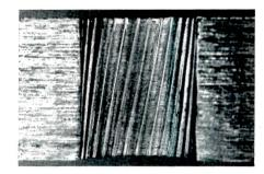
When driven, knurled bolts cold-work joint material, producing spiral-grooved holes
