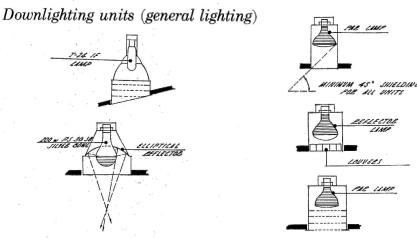
Control of light and direction are due to very accurate (external) reflector control built into the fixture itself
