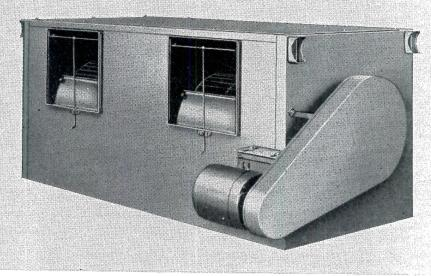
Multi-Zone H & V Unit — Type VB provides individual zone control of temperature from a single central unit. Utilizes a "blow-thru" arrangement with individual zone dampers at the discharge end. Typical applications: schools, laboratories, offices and stores. Bulletin 8927.
