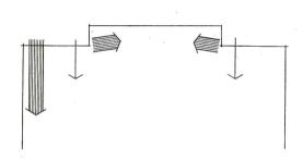
Downlights and washes again counterbalance uniformity of light from large luminous elements—in this case, indirect coffers
