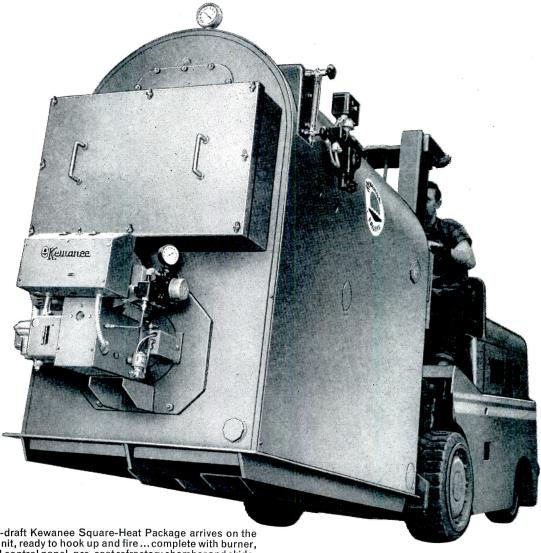
Forced-draft Kewanee Square-Heat Package arrives on the job as a unit, ready to hook up and fire... complete with burner, pre-wired control panel, pre-cast refractory chamber and skids. It requires no crating...no job-site insulating.
