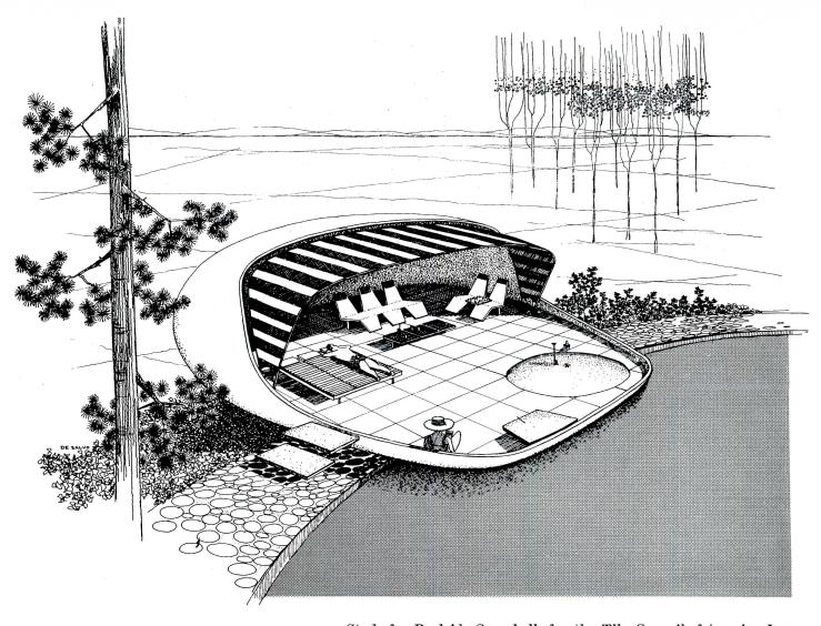
Study for Poolside Sun-shell, for the Tile Council of America, Inc. Designed to be built of the same materials at the same time as a sprayed-concrete pool
