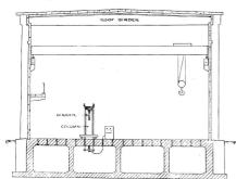
steel rods are attached to the object under test, extended through holes in the floor, and attached to jacks underneath it. Test loads are applied by the jacks, which can exert a total force of as much as 2 million pounds on a 50 ft beam.
