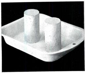
To compare the durability of Brixment mortar and ordinary cement-and-lime mortar, make a cylinder of each, let them "cure" for a month, then freeze and
