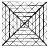
Latticed steel girders form folded slab, act as ring ties between diagonal ribs
