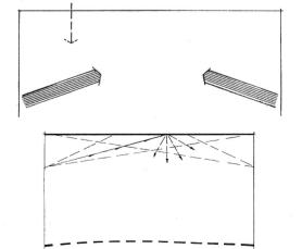
CEILING WASH. Directly lighted, high brightness ceiling reflects light to floors and walls, which have relatively low brightness. Lighting is diffuse in quality, almost linear in distribution
