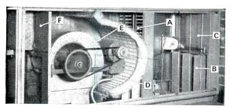
Lennox Air Processing Unit introduces fresh air in adjustable volumes (A); transmits warm air (B) from adjacent or remote heating unit; continuously recirculates indoor air (C); filters air clean (D). Lennox' exclusive floating blower (E) and acoustical lining (F) assure a degree of quietness never before achieved.
