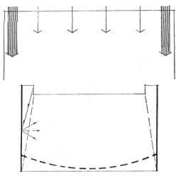
WALL WASH. Walls are high brightness elements; floor and ceiling, lighted indirectly, have low brightness. Lighting is diffuse, but downlights add contrast, modify light distribution curve shown
