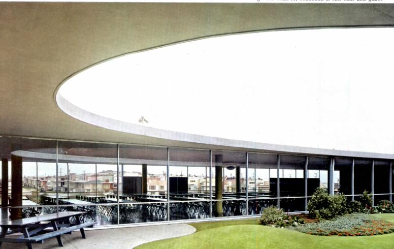
Cafeteria (viewed here from an inner court) has window walls of L·O·F Heat Absorbing Plate Glass for reduction of sun heat and glare.
