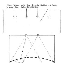
DOWNLIGHTING SYSTEM. Essentially a high contrast situation with relatively high brightness at floor. Walls and ceiling have low brightness level; objects are sharply defined highlights
