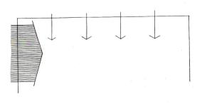
LUMINOUS WALL may become dominant element of design, must be carefully controlled to avoid excessive brightness and glare.
