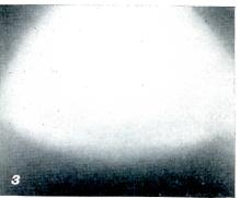
LIGHT DISTRIBUTION TEST: (1) Lens Panel: note how light is refracted away from the direct glare zone (dark areas) to heavy beams of light in the reflected glare zone. (2) Diffuser Panel: note how it evenly distributes light in the reflected glare zone but leaves a concentration of light at the high angle or direct glare zone. (3) Fiberglas Panel. note how light is reflected away from the direct glare zone by polarizing action and is evenly distributed into a soft diffused lighting pattern.
