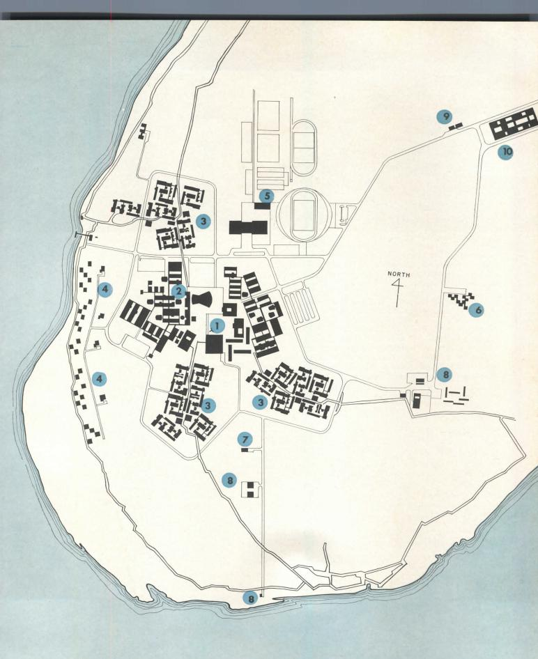
The site on the shore of the Tigris River is flat except for existing 10-ft high dikes indicated on plan by heavy irregular lines. These contribute a change of level within the campus. Two large groves of palm and fruit trees (not shown) determined the location of the central building complex. 1. Campus Center 2, Teaching Space 3. Student Residential Groups 4. Individual Housing 5. Sport Facilities 6. Elementary School 7. Infirmary 8. Service Facilities 9. Entry 10. Shopping Center
