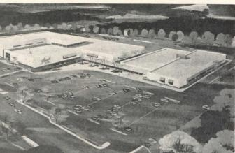
Two examples of two-level parking. At top, parking adjacent three separate entrances; bottom, the splitlevel plan arranged so the strips in front are filled first, giving the center an active look. Overflow parking in both cases is at the rear. Top: Lord & Taylor, Milburn, New Jersey. Bottom: Stewart's, Baltimore, Md.
