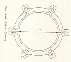
Phoenix Columns were formed by riveting together four, six or eight wrought iron segments, depending on diameter needed
