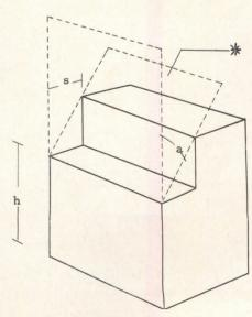
h: Height of sky exposure plane above street line; s: Initial setback distance; a: Angle of slope of sky exposure plane over zoning lot measured down from the vertical; \*: Sky exposure plane
