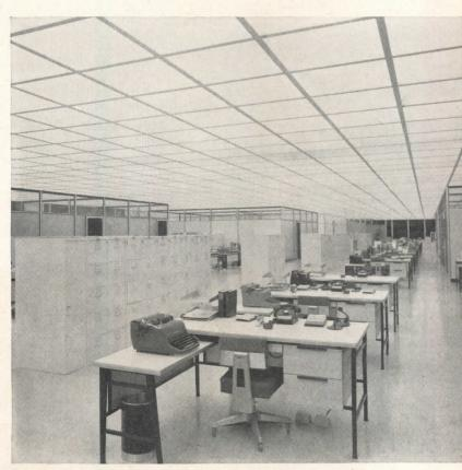
■ Large office areas are as effectively illuminated as small areas with a high degree of visual comfort assured. In this special Curtis grid installation, aluminum materials were used throughout. Maintenance features of the system include ease of relamping, ready access to wiring, and simple replacement of the ballasts.
