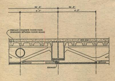
Structural steel frame of Shell building is sheathed in aluminum; spandrels and mullions are also of aluminum. Enclosing walls are of heat-reducing gray glass. Plan (opposite page, top) at building corner shows mullions set on every other module; partitions can be set on any module, with filler panel to glass on modules between mullions. At left: section and structural plan
