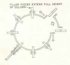
Vertical filler pieces between flanges of "Improved Phoenix Column" added to rigidity, ease of making column-beam connections
