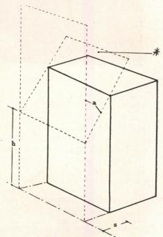
h: Height of sky exposure plane above street line; s: Depth of optional front open area; a: Angle of slope of sky exposure plane over zoning lot measured down from the vertical; \*: Alternate sky exposure plane
