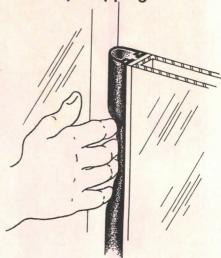
The ZERO weather stripping #72, with its flexible looped neoprene incorporates a safety feature. Protects fingers from being crushed between the door and jamb; or between pairs of doors when used as a meeting stile. This equipment is recommended for public buildings.
