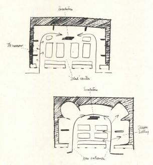
Above, an unfortunate (top) and improved (bottom) diagram-plan for the placement of entrances and their working relationship with internal circulation, as well as the size and shape of selling areas in conjunction with both
