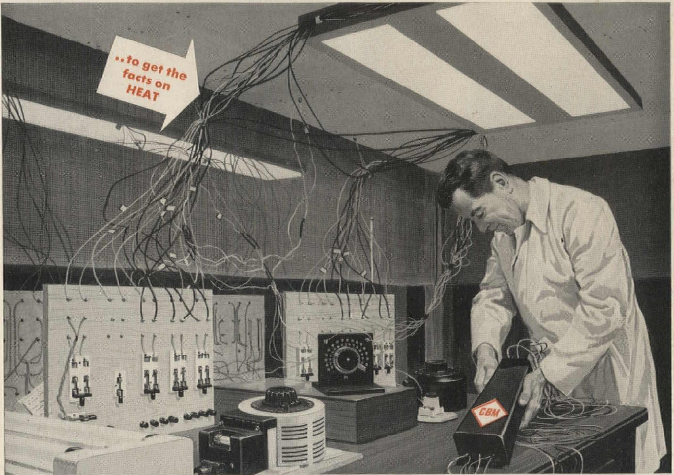
This maze of wires above is needed to connect with thermocouples in fixtures, ballasts and other parts, so temperatures can be measured at different points. Screening shields break up drafts from air conditioning, help keep ambient constant.
