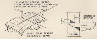
The final scheme was based on a notched column, with a rigid arch extending into the column. A check on bearing stresses at top and bottom of the notch gave a satisfactory solution
