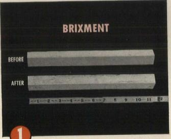
In these autoclave tests, the bottom bar in each set of neat cement bars above was exposed to 295 lbs. steam pressure, 420° F., for 3 hours. Left: The two bars are both Brixment. Note that it
