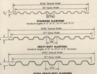
EXTRA HEAVY-DUTY SLABFORM and Lengths: 6'-0" to 21'-6" in 6" Increi
