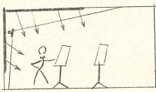
Figure 4 vertical lighting from wall on ceiling
