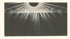
recting the light downward away from the line of sight, objectionable glare is avoided. Troffers at Equitable have reflectors above lamps so that lens-prisms receive and re-direct all light available. Holophane Co., Inc., 342 Madison Ave., New York 17, NY
