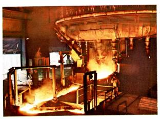
Tapping molten iron from a blast furnace
