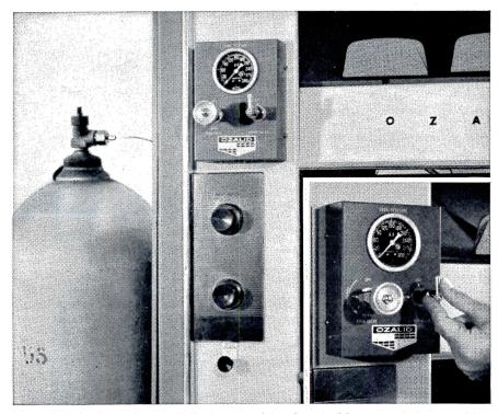
Ozalid® Anhydrous Ammonia System consists of control box mounted on machine and tubing to connect equipment with anhydrous ammonia cylinder, which may be remotely located. Developer handling becomes simply, "valve on, valve off."
