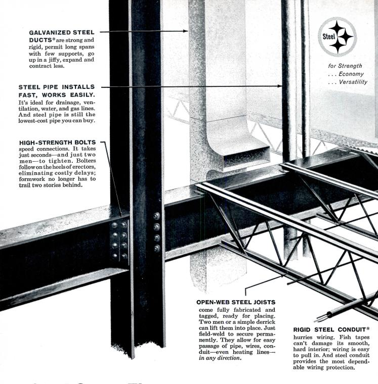
**Steel Saves Time** Shop-fabricated structurals and Bethlehem steel joists arrive ready to go up. No falsework, no delays because of weather. Long before the frame is completed, other trades can move in and get started. You can make—and keep—a completion promise when you build with steel.
