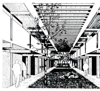
Malls are glass enclosed at the roof, and will be partly heated by radiant panels in the soffit of the walkways during the winter months
