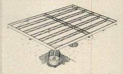
to accommodate the legs. The perimeter has four 12-gage galvanized "C" members. Exterior beams are further protected with coal tar. The perimeter beams rest on four corner posts and eight intermediate posts. Concrete is poured around bottoms
