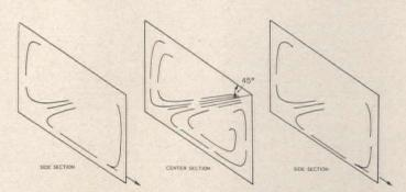
Figure 4: End-wall grille air distribution, 45 per cent inlet
