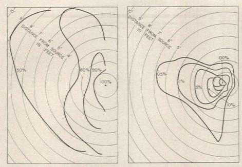
Figure 8: Distribution of settled bacterial particles for perforated ceiling (left), no mechanical ventilation (right)
