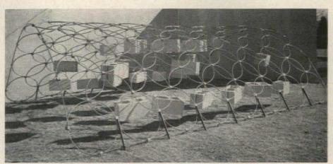
Concrete blocks suspended from this model of the "Aluminum Curvilinear Truss System" designed by Manuel Fernandez demonstrate its load carrying capacity
