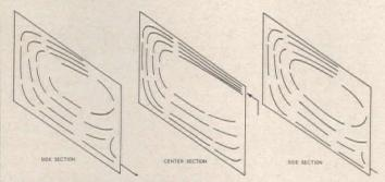
Figure 3: End-wall grille air distribution
