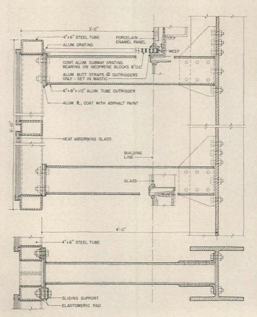
A solar- and glare-reducing screen of tinted glass which surrounds the Municipal Office Tower of the Norfolk, Virginia Civic Center will cut heat gain sufficiently to make the glass facade between spandrel beams equivalent to a wall of 53 per cent glass and 47 per cent 12-in.-thick masonry.
