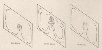
Figure 6: Central diffuser air distribution, vertical
