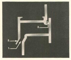
Triple Weather Guard—1) Pressure equalization slot, 2) integral drip, and 3) neoprene weatherstrip. The Sealair window offers triple weather protection. Weathering where needed, scientifically designed.
