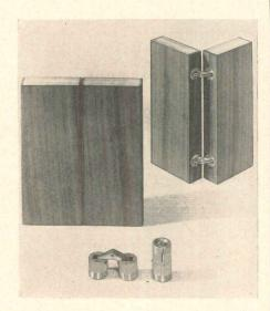
hinging action, the hinge works equally well on flake-core, chip-core, lumber-core and solids. The hinge is made of solid brass with heavy steel linkage and can sustain heavy loads. Two primary uses are on flush door cabinets and house doors. The hinge, *Model No. 610*, comes in four standard sizes, from 14 to 24 mm. *Selby Furniture Hardware Co.*, 17 E. 22nd St., New York 10, N.Y.
