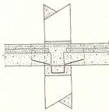
Beam and girder connection (at interior columns)
