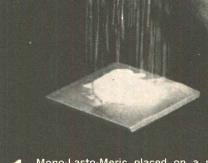
Mono-Lasto-Meric placed on a metal plate, allowed to set a few minutes to skin over, then sprinkled lightly with "construction dust" to form a typical deterrent to good construction joint
