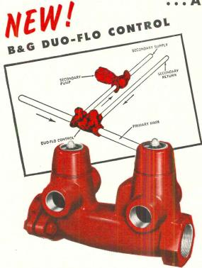
In primary-secondary systems equipped with Duo-Flo Controls, secondary zones are always controlled, even with high head pumps in the primary zone. Use of higher temperature drops permits sizable reduction in pump horsepower. Material saved includes 2 Flo-Control Valves, 2 shut-off valves, 2 or 3 tees and 6 nipples.
