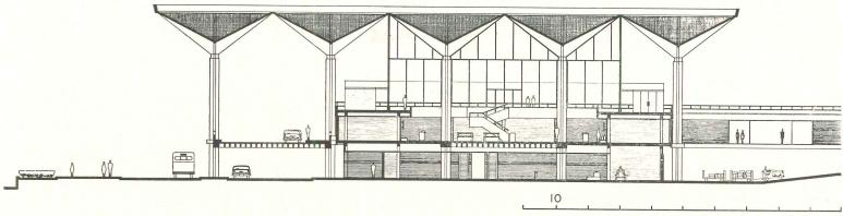
Section through terminal including apron level, main passenger floor, concourse bridge and mezzanine
