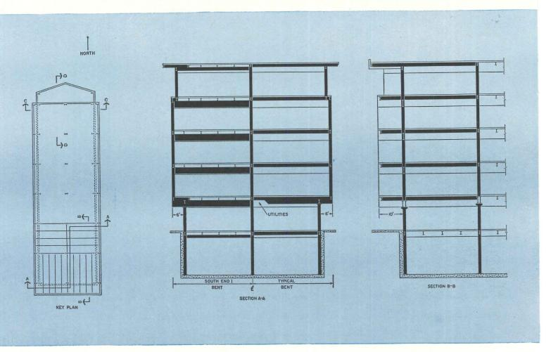
In the unique design of the Allentown City Hall and Police Building, the main tower is cantilevered at the second floor on three sides—6 feet on the east and west, and 10 feet on the south.
