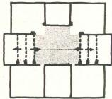
INTERMEDIATE FLEXIBILITY: Folding partition moves to dashed positions by shifting
