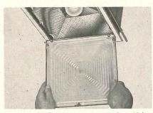
New removable door design permits entire door with lens to be removed easily for cleaning; but it can not accidentally fall out of fixture. This latter is very important with pole relamping, as is the accessibility of the vertically mounted lamp in No. 1611VY-T. (Removable door is standard on most models).
