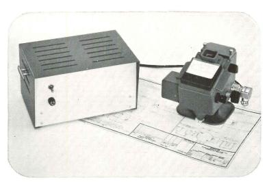
New Microline Evaluator—Makes every microfilm near-perfect and eliminates retakes. It assures complete legibility of all microfilms, permitting blowbacks to original sizes with absolute minimum loss of detail. Microline® Evaluator measures reflectivity of lines from .005 inch. Prominent suppliers of microfilm to the military believe this instrument will bring about a change in the MIL-STD specifying microfilming requirements.
