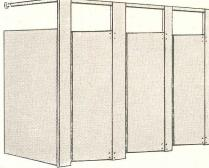
Wall Hung Hi-Stile features overhead bracing.
