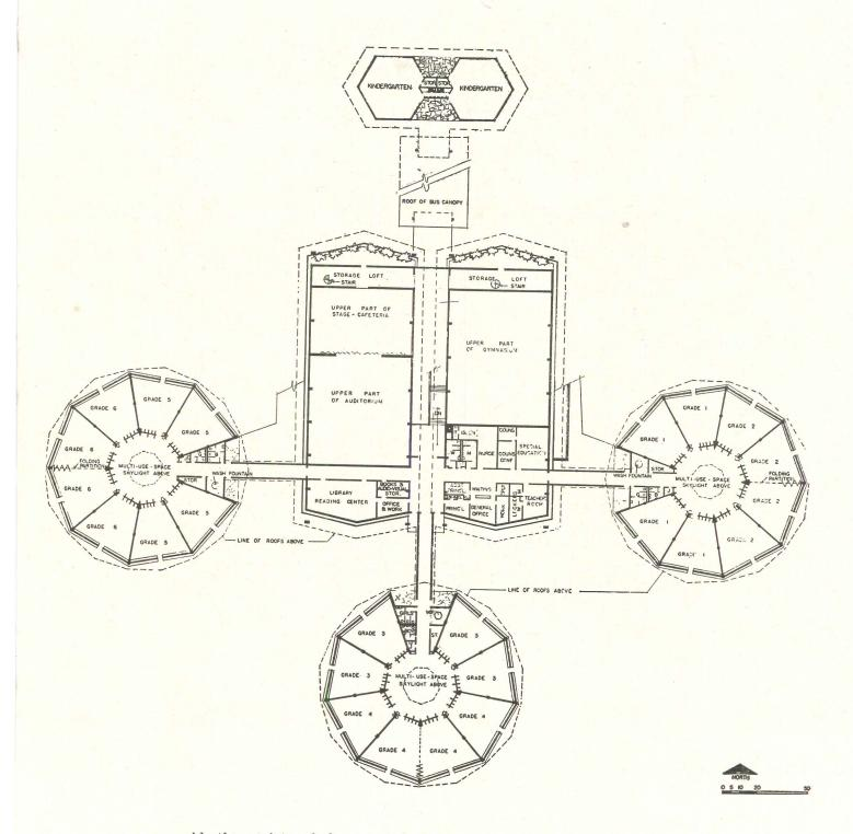
provide the variety of classroom shapes for team teaching, dividing walls are non-load bearing and contain no utility lines, and can be easily replaced by folding partitions. In the meantime, multi-use corridors in the classroom wings, and the large spaces in the central building, are available for a partial program."
