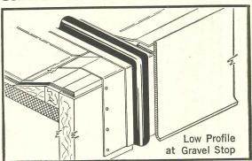
Typical Roof Expansion Joints
