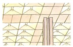
Modifications to fit under beams and around columns. Whether the main structural members are parallel with the fluorescent tubes or perpendicular to them, the modification is the same: a row of flat ceiling panels replaces a row of regular Luminaire modules. This creates a space wide and deep enough to accommodate the beam. The flat panels rest on the Luminaire Ceiling grid.
