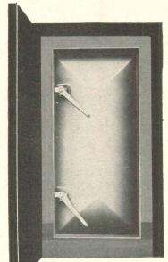
Safety from shock and pressure—Using a concave-convex design, the Overly blast-resistant door is engineered in two models to resist pressures up to 10 atmospheres or 147 pounds per sq. in. (Model 10 atü) and 3 atmospheres or 44 pounds per sq. in. (Model 3 atü). Man-sized escape hatches are available with identical ratings. Lower rated doors at 2.5, 6 or 10 psi overpressures are regularly manufactured by Overly in more conventional flush 13/4" design.
