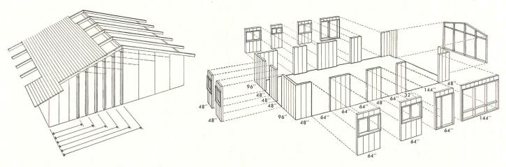
UNICOM's plank-and-beam roof is readily co-ordinated with modular dimensions. Loadbearing walls and columns, in some of these designs, can vary the wall components.
