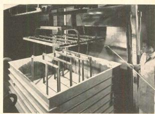
Steel window frames being dipped in tank for coating by fluidized plastic process
