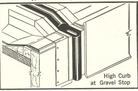
... The Metal Water Stop with the Flexible Neoprene Bellows for Expansion Joints
