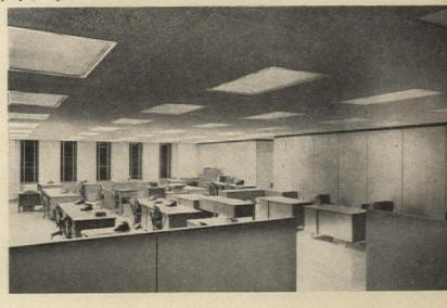
Window spacing on typical floor (shown in plan at left and photo above) is based on minimum office space requirements. Lighting levels range from 100-200 footcandles, depending on the type of work. On the 12th floor the fenestration module changes and reflects special uses. The exterior walls enclosing an auditorium on this floor are unbroken by windows, and those surrounding a lounge consist of large panels of glass divided by slender mullions
