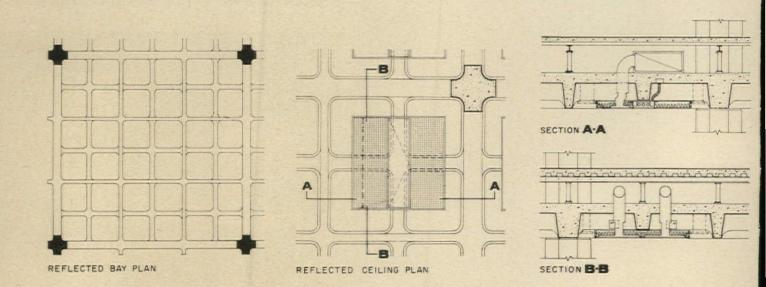
Every effort was made to design using natural materials and to create an integrated structural, mechanical and electrical system that would permit the structure to participate in the interior spaces. An exposed sandblasted concrete column and dual depth waffle slab structural system with the mechanical space above the slab permitted the concept to be fulfilled. Separation of floors and mechanical spaces by concrete also greatly reduces noise transmission problems.
