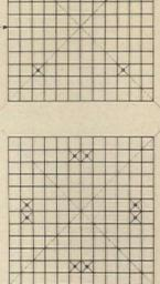
Structure *left* is a three-dimensional Warren truss system supported at four points. Two-way vertical trusses are used in system *right*  Various column arrangements give axial symmetry. It should occur about two, preferably three, axes
