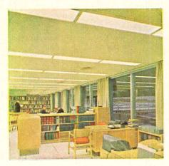
At the new 3M Company Administration Building in St. Paul, lighting of the highest quality is obtained through nearly 11,000 control lenses injection molded of PLEXIGLAS® acrylic plastic. Each lens is a single, precisely designed, four-foot molding that provides a high level of directed light with minimum surface brightness.
