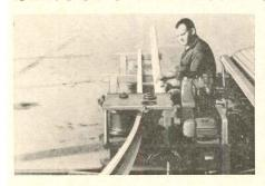
Self-supporting sheet metal arches spanning up to 40 ft with 30 lbs per sq ft live load can be field assembled from 6-in.-wide, 2-ft-deep U-shaped steel sections, which are perforated for acoustical properties and have a baked vinyl enamel finish on the underside. The top of each leg of the U
