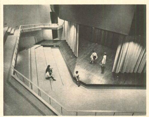
A theater is provided for the Drama Department at one end of the building, with adjacent work and teaching spaces. The building has a frame of reinforced concrete, and exterior walls of concrete and brick; the roof has shingles and built-up roofing.
