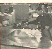
HIGH COVERAGE, MINIMUM HIGH COVERAGE, MINIMUM LABOR! Using 3M-recommended spray system, a gallon of Insulation Adhesive 33 effectively bonds about 600 square feet of duct liner. Open time of 5 to 7 minutes permits spraying large areas quickly, conveniently.
