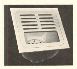
FLOOR SINKS / Enameled cast-iron floor sinks are designed for use in restaurant, kitchens and other establishments where sanitary, easy-to-clean drains are required. The drains are set in concrete flush with the floor and are said to be hard wearing and acid-resistant. American-Standard, New York City.
