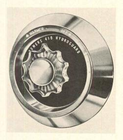
shower control / Protection from icy blasts or scalding bursts of water can be achieved by use of the *Hydroguard series 410*, which can sense and correct any fluctuations in supply water pressure. This new control, operating on the pressure-equalizing principle, incorporates a diaphragm which positions poppet valves to compensate for water pressure changes as they occur. The Powers Regulator Company, Skokie, Ill.
