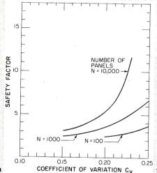
lights out of 1,000 would have a strength 42 per cent less than the mean. Figures 7a and 7b show how both the coefficient of variation and the total number of glass lights in the building change the required safety factor. With only a small number of lights, differences
