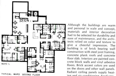
had to be selected for durability and ease of maintenance, and the architects relied on color and texture to give a cheerful impression. The building is of brick bearing wall construction with steel joist framing, concrete plank roofs and concrete floor slab. Interiors are painted concrete block walls and vinyl asbestos floors. Brick accent colors are used on the doors and other wall panels. Radiant ceiling panels supply heating and air conditioning. Food serv-
