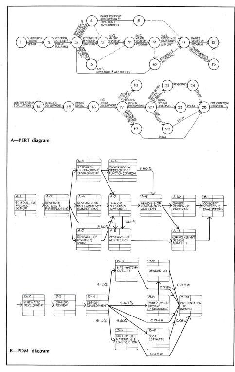
definition of tasks should be given as much thought and consideration as possible so as neither to belabor the diagram with an excessive amount of detail, nor to decrease the effectiveness of the diagram by being too brief. When a basic list of work items is assembled, it becomes a simple procedure to expand or delete from the list as necessary.
