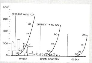
In open country the wind, obviously, will have faster velocities than in the built-up city. Graphs above (based on work by A. G. Davenport) show how the profiles of the wind vary with with the terrain "roughness."
