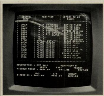
creen shows input form with the dimensional information for one wall filled in. A complete geometrical description of the entire building shell, and all major sub-areas such as doors and windows, is a necessary first step to this computerized cost analysis system. Descriptive process also includes certain basic information about the nature of the building, such as whether glass is fixed or movable, presence of insulation in the wall, and so on.
