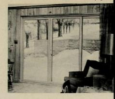
PATIO DOOR / Insul-Dor is reported to allow 81 per cent less air infiltration than the established standard. Polypropylene pile has been added at points of potential leakage and a vinyl insert for the sill helps prevent "wicking" of water. Wood members are reinforced by recessed metal which promises continued alignment, proper seal and easy operation. R.O.W. Window Sales Co., Ferndale, Mich.
