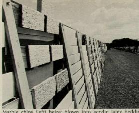
Marble chips (left) being blown into acrylic latex bedding test panels (above) show no adverse effects of weathering
