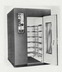
ENVIRONMENTAL ROOMS / An added 8-in. interior width to the V.I.P. fifty-si. controlled environmental rooms pro vides up to 25 per cent increase in load ing area, and up to 56 cubic ft of added chamber space over previous models The "Lumen-Aire" ceiling plenum serve as a combination air-conditioning and air-flow chamber and permits uniforn light transmission throughout the room Lab-Line Environeers Inc., Melrose Park, III.
