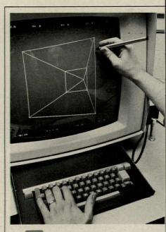
omputer graphic techniques may one day make it much easier for the architect to place a description of the building he is designing in the computer memory, as he will be able to draw it directly on the face of a cathode ray tube by means of a "light pen." Cost figures could then be related to purely graphic descriptions of the building, giving the designer even more immediate access to the cost effects of new dimensions or configurations.
