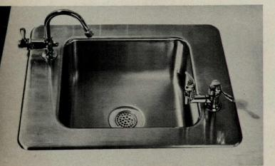
Classroom Counter-Top Fountains Complete "self-rimming" type pre-assembled for easy installation. Stainless steel receptor has push-button-operated, two-stream projector with automatic stream control. Goose neck glass-filler faucet optional. Also available in porcelain-enameled cast iron.
