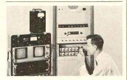
FILTERED ACOUSTICS / A technique called Varacoustics uses small filter networks, custom-installed to control sound regardless of room acoustics. The system is said to assure that a professional quality sound system will perform with high fidelity in any large audience enclosure. DuKane Corporation, St. Charles, Ill.
