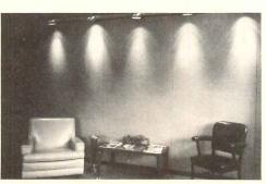
BURLAP BOARD / The base of standard 15/32-in. insulated board is surface-laminated and long-edge wrapped with tightweave, natural color, all-jute burlap. The surface may be used for an entire interior, an accent wall or for many other uses. Homasote Company, Trenton, N.J.
