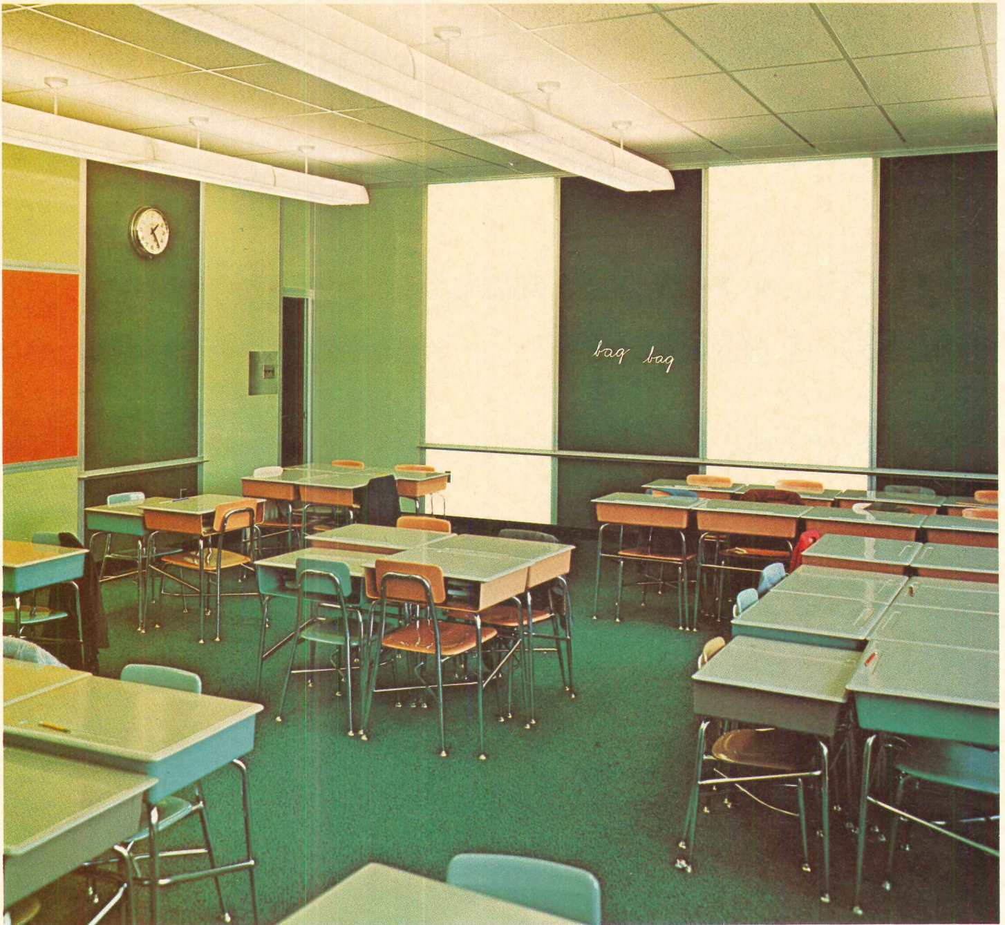
Here forest green and feltwhite 118 chalkboards are extended to ceiling to bring extra color and brightness to classroom. Magnetized chalkrails can be raised or lowered and removed for projection of films.
