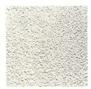
Conwed "Rough" Rock Face, a deep, naturally textured, white surface pattern; <sup>5</sup>/<sub>8</sub>" thick panels 24" x 24" or 24" x 48".
