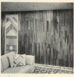
**ELEMENT I** includes basic designs that encourage distinctive interiors. Palisades (left) is created with U-shaped profiles that support the illuminated ceiling and act as a background for the desk. In Ionic (above) highly figured veneers alternate with reveals. Butcherbloc (top right) is a random pattern inlaid in vertical rows. And Collage has veneers of varying lengths and widths that overlap vertically and horizontally. U.S. Plywood, New York City.
