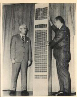
CENTRAL HEATING-AIR CONDITIONING / Hydrowall is a total gas energy combination air conditioning and recessed wall furnace designed to provide year-round comfort for as many as four rooms without requiring duct-work. The unit, which is developed for apartments, motels, offices and residential applications, may be installed freestanding or it may be partially or fully recessed in the wall.
