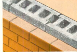
2 For non-aligning horizontal joints.
