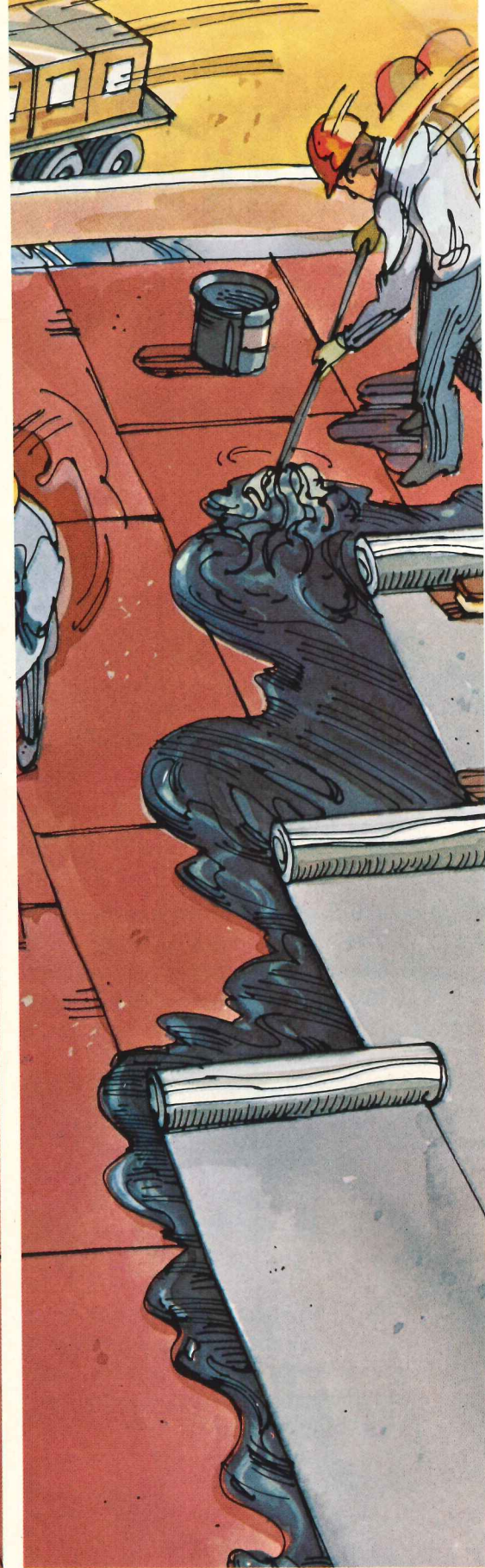
J-M Centurian® Asbestos Base Felt.
