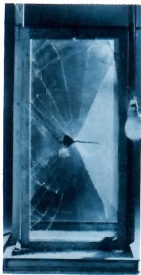
WIRED GLASS. This type of glass breaks similarly to traditional glass with the bag passing through the wire net—Shards with jagged edges surround the hole but more pieces of glass stay in place around the point of penetration. Cut wire protrudes.
