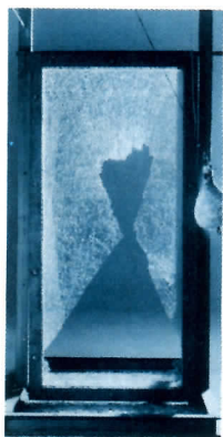
TEMPERED GLASS. This type of glass requires a higher impact energy to break. When it breaks, it shatters completely and the bag passes through it. Only a small number of glass pieces remain in the frame.
