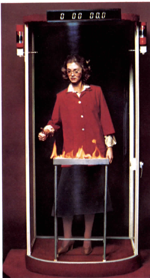
1. Flammable liquid ignited. Halon 1301 cylinders discharged.
