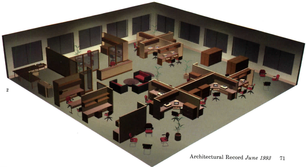
The wireless-frame image (1) grew out of a 2-D AutoCAD floor plan. It was rendered in 3-D Studio and saved in Adobe Photoshop to produce image at right (2). Note the video-captured landscape through the windows in the more detailed closeup above (3).
