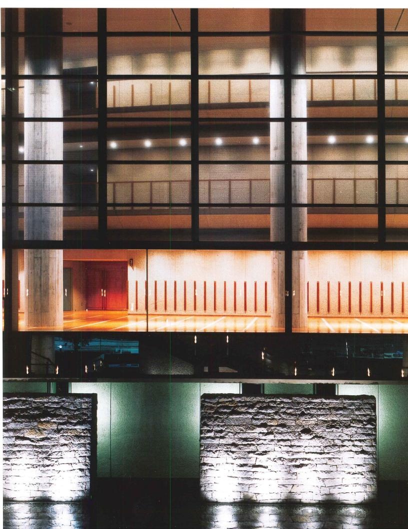
A view across the reflecting pool (opposite) to the foyer outside the opera house shows how different planes are lit to create numerous layers between the interior walls and the exterior of the building. A view from within the foyer (below) shows how the columns are washed to give them a greater sense of depth.
