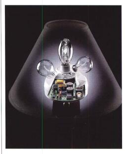
Microsun uses a pair of 15W incandescent lamps to provide illumination during the 30 to 45 seconds the miniature metal-halide lamp needs to warm up. An electronic ballast powers the device.
