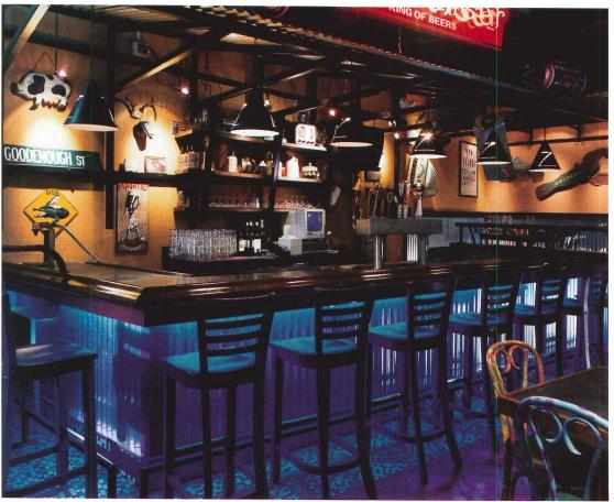
The message Doreen LeMay Madden wanted to communicate with the layers of light in this replica of a tacked-together bayou bar is the same as that of Zydeco music: have fun! The underside of the bar is lined with intense horizon-blue neon, and the bar has custom pendants overhead. The walls, which are decorated with Louisiana artifacts, are bathed in light by a track of MR16s over the back bar.
