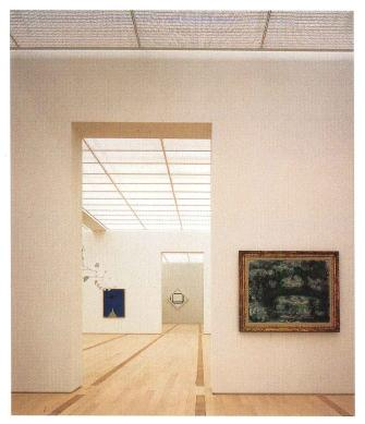
and the dramatically projecting roofs at the Beyeler. The transparent glass-panel roof system uses photovoltaics and motor-driven louvers to guide overhead daylight into the galleries in a natural way while keeping light levels within strict curatorial criteria (targets of 80 lux for works on paper and 50 to 200 lux for oil paintings).
