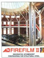
Improved spray characteristics and ratings up to 3 hours! A/D FIREFILM®II permits designers to use the appearance of exposed steel with the steel protected from fire. The product is applied as a thin-film coating 0.4 to 3.3 mm (16 to 130 mils) thick. When exposed to fire it expands to form a meringue-like insulating layer up to 4 in. thick. A/D COLORCOAT topcoat is available in a wide range of colours. Call 1-800-263-4087 or 416-263-4087. Internet: www.adfire.com
