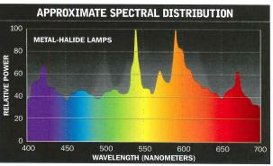
The spectral distribution of high-pressure sodium (far left) is very low in blue but comparatively rich in red and yellow. Metal-halide light (left) contains a much greater quantity of blue.
