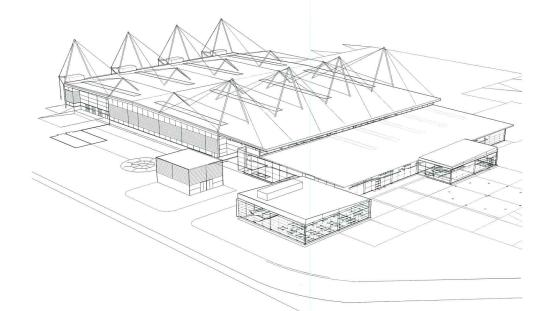
Eliminating columns in the fabrication area made the space more flexible, but it also necessitated the dramatic fretwork of columns and tension rods that make the truss system so striking.
