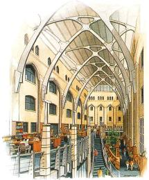
Yale University is filling a courtyard in the 1930 James Gamble Rogers Sterling Library with its music collection. Shepley Bulfinch Richardson and Abbott's design allows indirect light (above). The neo-Gothic trusses were designed in components that could be bolted together at the base of the court.
