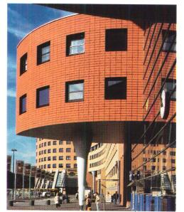
new station. All of the massive building elements are hidden behind an Argeton clay-tile facade, which conveys an impression of lightness. The archshaped design of the facade lining was made possible by the small size of the panels. Patented in Germany in 1984 by Möding, Argeton was introduced in the United States last September exclusively through Shildan U.S.A. Inc. Available polished.
