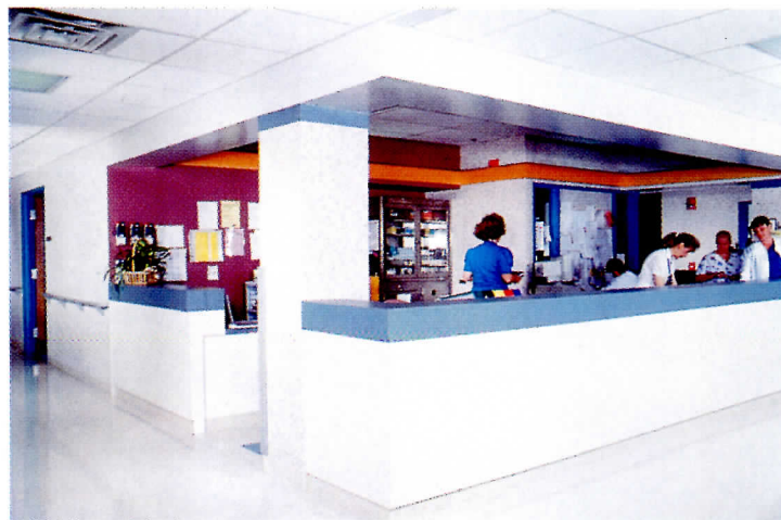
In a health-care facility, there's no opportunity to close down operations and paint the walls. Specifiers must select fast-drying, low-odor latex formulations that stand up to a lot of traffic.
