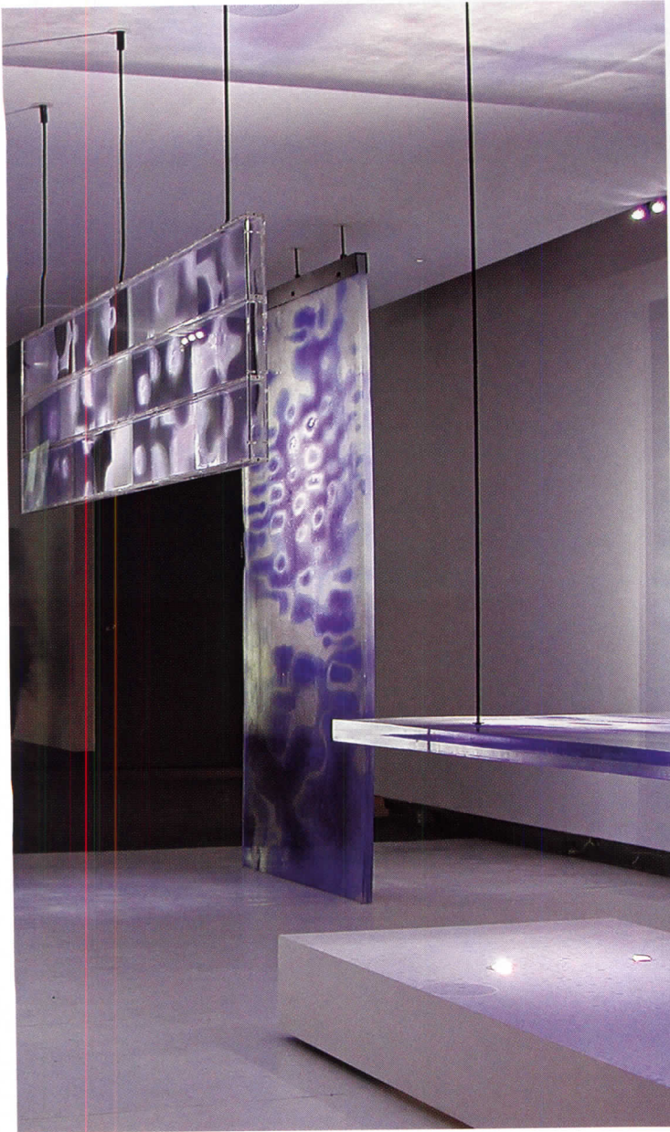
Cast-resin panels of aerogel tiles (left) demonstrate the latent architectural potential of a highly effective insulating material.
