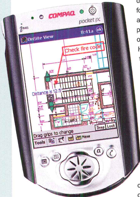
PocketPC devices, such as the Compaq iPaq, which use Microsoft's WindowsCE operating system, are especially well-suited to running CAD programs like Autodesk's OnSite View.
