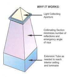
the tube down or horizontally into building interiors. Tubular skylights can provide high quality light with little heat or glare. They are useful in areas that are difficult to light, and in buildings that have special lighting requirements, such as laboratories and museums. They can also provide "skylights" for the lower floors of multi-floor homes or buildings.
