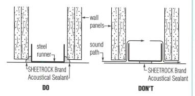
Sealing flanking paths in wall partitions is a critically important factor in controlling transmission. An adequate bead of acoustical sealant should be applied to both outside edges of the floor, ceiling and intersection tracks (left).
