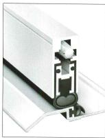
Tested through 5 million cycles, they are engineered for easy, precise installation, with a minimum of parts subject to wear. Quality construction to renowned ZERO standard makes these gaskets the choice for superior performance & unequaled service life. Double neoprene seals & a patented spring action, automatically drop & retract in a scisor like motion as door is operated. 800-635-5335 or 718-585-3230; FAX 800-851-0000 www.zerointernational.com
