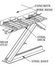
ductwork can run through the open webs of the joists. And the system is almost always less expensive than cast-in-place reinforced concrete construction.
