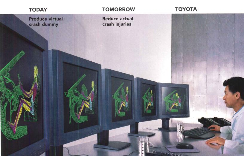
He can't talk, he can't walk, he can't drive a car. Yet he could be the most important "person" in the world of automotive safety testing today. He's THUMS, the world's first virtual human for crash testing.
