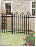
Monumental Iron Works™ is a modular system with the solid look & feel of authentic wrought iron. When assembled, it creates one of the strongest ornamental fence systems on the market. Welding processes are eliminated to avoid red rust problems. MIW utilizes a duplex coating of polyester resin over hot-dip galvanized steel for corrosion protection. Master-Halco, Baltimore, Maryland 21040. 410.676.2744 Email: spec@fenceonline.com Web site: www.fenceonline.com
