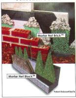
Mortar Net invented the mortar dropping collection device for brick masonry cavity construction and single wythe concrete masonry units (CMU). By breaking up mortar droppings, Mortar Net for brick and Mortar Net Block prevents mortar debris from forming a barrier against water flow to the weep holes thereby eliminating moisture damage to masonry walls. For more information call 800-664-6638 or www.mortarnet.com.
