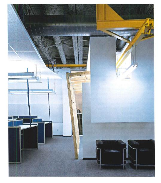
Remnants of the toolmanufacturing process, such as the yellow ceiling tracks and hoists, were incorporated into the new office design (right). Fluorescent pendants, once used to downlight the assembly line, were retained but rehung upside down to provide ambient uplight above the work cubicles for phone operators (right and below).
