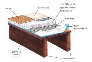
Acousti-Mat\* 3 is the sound deadening solution for floor systems that have been impossible to control! Put an end to those "noise" complaints — even with open beam, concrete slab and conventional wood frame systems. Maxxon Underlayment is poured over the Acousti-Mat 3, resulting in a 15 IIC rating point improvement over conventional wood frame or open beam construction!
