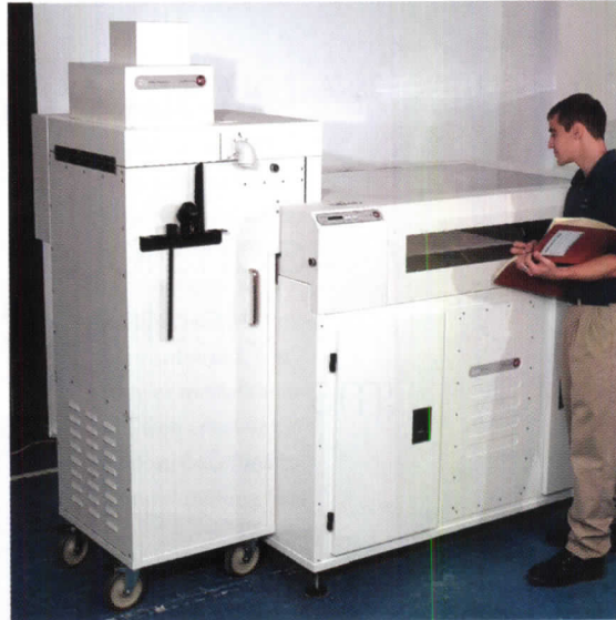
Z Corporation makes 3D printers for creating physical prototypes from CAD drawings. The Z810 System is shown here.
