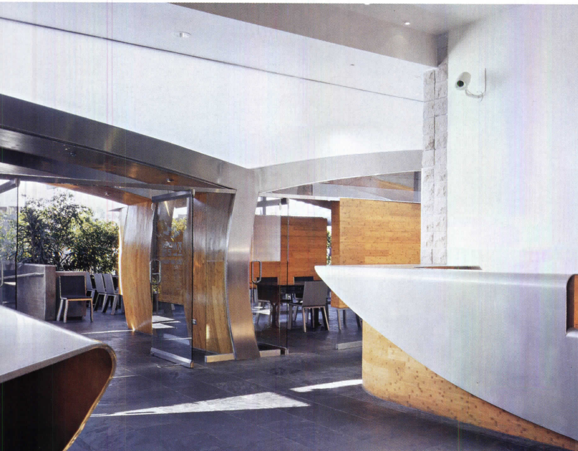
The reception area and bar tops (left) are covered in aluminum plate, while the floor is honed slate. Stainless-steel hoods are the dominant design motif of the main dining area (opposite, top); while bamboo-wrapped steel arches and bamboo-screen walls in the private dining rooms afford privacy with views out (opposite, bottom left). Rolled-steel beams form a pergola over the outdoor dining area (opposite, bottom right).
