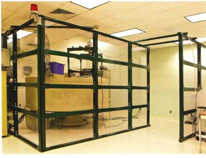
The centrifuge at the Department of Energy's Plantex Plant is protected by an enclosure made of the Unistrut structural metal framing system. The enclosure uses standard 4-by-8-foot polycarbonate bolted into U-channels.
