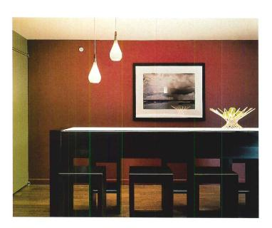
effect is grazed by T8 fluorescent strips fitted with color sleeves moun in a cove above. A rectangular ceiling cove with knife edges is lit with d blue neon, creating the illusion of an endless night sky overhead.
