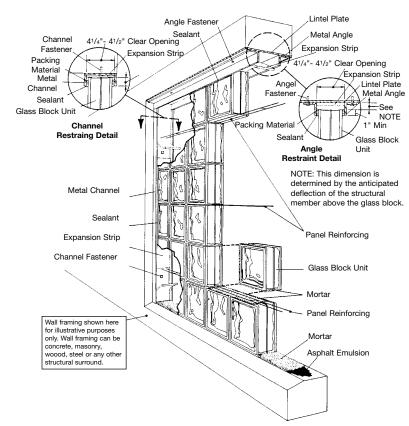
The unit can be hollow or solid and come in a variety of sizes, shapes, patterns, and textures. The most commonly used units are square (6-, 8-, or 12-inch sizes). Rectangular units (4x8-inch and 6x8-inch) are also available, as are bull-nosed edge blocks for finishing horizontal and vertical panels, and various corner and angular blocks.
