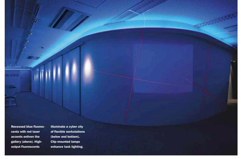
high-output (1,000 lux) blue fluorescents and mini-halogen pinlights illuminate the general work areas. Each workstation is also lit by a clip-mounted lamp designed by Tolomeo Pinza.
