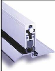
Automatic door bottoms, designed & built to last. Tested through 5 million cycles, they are engineered for easy, precise installation, with a minimum of parts subject to wear. Quality construction to renowned ZERO standard makes these gaskets the choice for superior performance and unequaled service life. Double neoprene seals and a patented spring action, automatically drop and retract in a scissors-like motion as door is operated. Fax number 800-851-0000.
