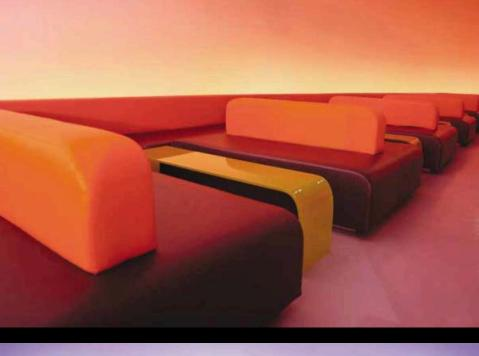
Lighting the back wall, striplights behind the banquettes produce an even wash of light from floor to ceiling (left and below left). Colors shift in gradual fades. Mounted below risers, T8 fluorescents with color sleeves add sparkle to the bar (below right).
