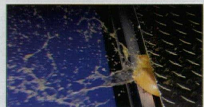
Actual demonstration of the closing force of a "lift assisted" non-Bilco floor door
