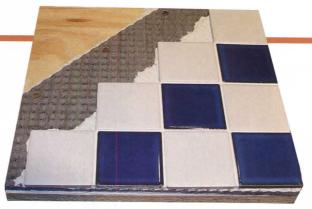
Nybacker tile backer-board uses postconsumer and postindustrial recycled carpet which, unlike cement-based backer board, does not release silicon dust when it is cut. The board features a rough surface with indentations for tile adhesion on one side, and easily affixes to plywood on the other. Nycore, Atlanta. www.nycore.com CIRCLE 202
