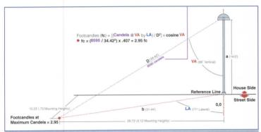
Figure 3: Footcandle representation based on Candela Tabulation Data
