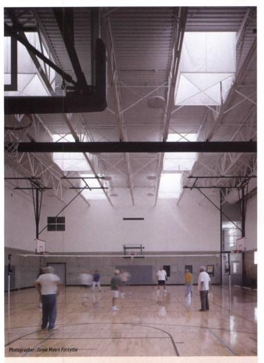
Southwest Community Center Gymnasium, Seattle, WA: This gymnasium uses fabric skylight baffles to diffuse glare and make electric lighting unnecessary during daylight hours. Architect: Weinstein AlU
