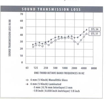
A PVB interlayer increases glazing Sound Transmission Loss (STL) without significantly increasing the glass thickness or mass of a glazing system.
