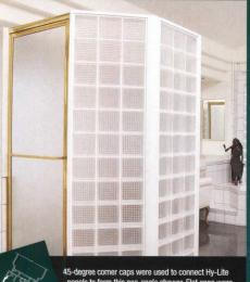
45-degree corner caps were used to connect Hy-Lite panels to form this neo-angle shower. Flat caps were used to finish off the top and sides of the doorway, while a flat cap and mounting channel were used to attach the panels to the curb and wall.
