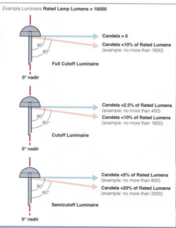
Figure 6: Definitions of Cutoff Luminaires
