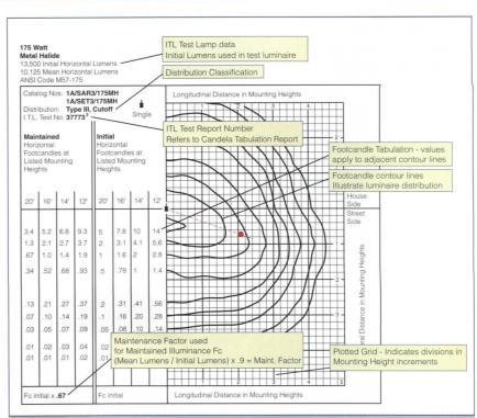
Figure 7: Elements of a typical Isofootcandle plot
