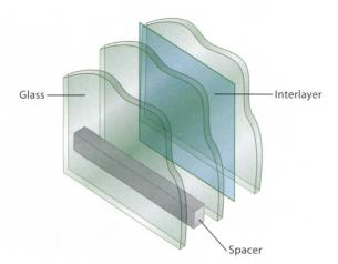
PVB is the main component in laminated glass. The fused interlayer and glass function as a single unit and can be used in almost any configuration. Used in an insulating glass assembly (pictured above), laminated glass can help improve the thermal and sound-reduction performance of a glazing unit.
