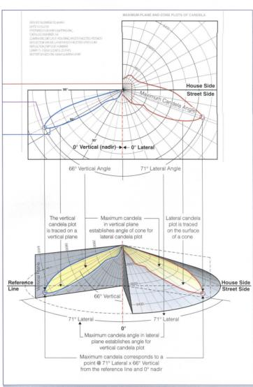
Figure 4: Maximum Plane and Cone Plots of Candela
