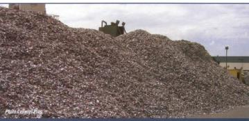
About 18 beverage cans are recycled per square foot of aluminum ceiling. Used cans and other scrap are taken to local reclamation plants where they are shredded, melted, formed into ingots, and rolled into sheets. Since a relatively small amount of energy is necessary to melt and reuse aluminum, aluminum ceilings have only low entrained energy
