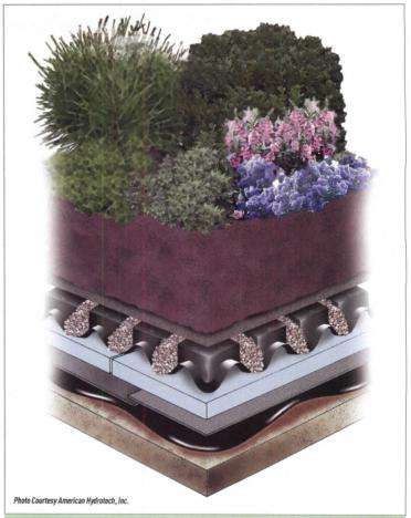
Assembly of Intensive Garden Roof.
