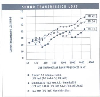
A This figure presents a comparison between two 25.4mm (1 inch) insulating glass configurations, one using two lites of 6mm (1/4 inch) monolithic glass and the other using two lites of 6mm (1/4 inch) laminated glass (LAG). The 6mm (1/4 inch) laminated glass consisted of two lites of 3mm (1/8 inch) monolithic glass laminated together with 0.76mm (0.030 inch) PVB interlayer. As a reference, the STL for 12.7mm (1/2 inch) monolithic glass is provided.
