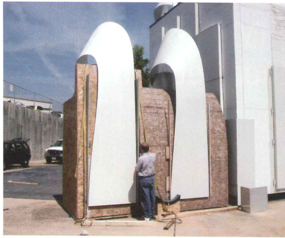
The High's designers built a mock-up of the skylight sunshade to identify any weaknesses inherent in the sail-like shape.
