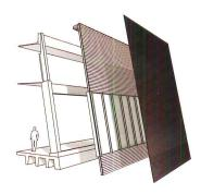
it, too," Trahan says, creating a patchy look. After lots of testing, he found an aluminum panel and a chemical bath to give it the correct patina—that provides a whole new skin for only \$200 million. Panels will affix to the surface without rivets, allowing repairs. Construction will begin in 2009. Alec Appelbaum
