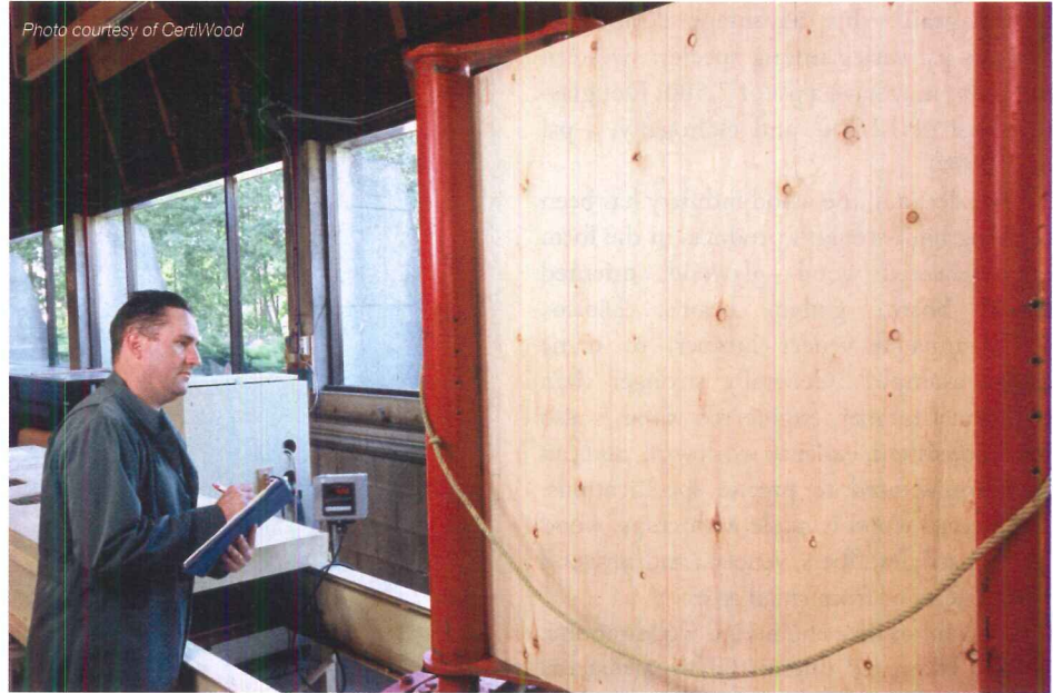
Flexure test machine for testing full size panels for bending movement and stiffness
