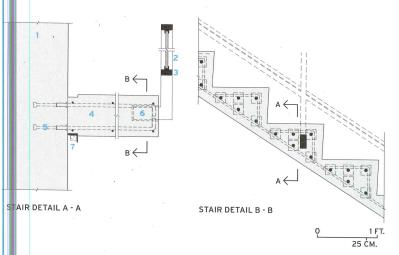
CONCRETE WALL GLASS PANEL STEEL HANDRAIL CONCRETE TREAD FORM SAVER FOR TAIR REBAR STEEL SLEEVE FOR HANDRAIL UPRIGHT .ED LUMINAIRE
