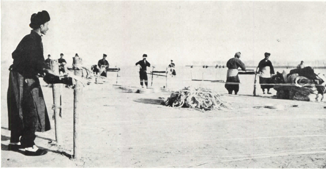
EVERYTHING ON THIS JOB WAS HOME-MADE. Hemp from nearby farms is hand-twisted into three-strand rope in a method almost as old as the river itself.
