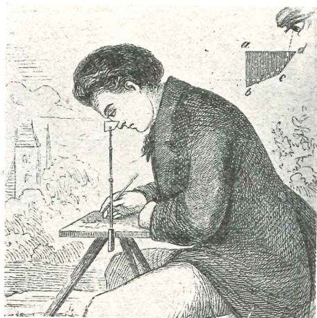
End of 18th century. Camera Lucida. A mechanism with prism which projects a view onto the drawing board. The picture is then traced
