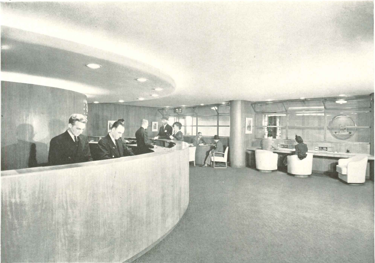
A semicircular false ceiling over the tellers' counter is intended to give an illusion of greater height to the room.
