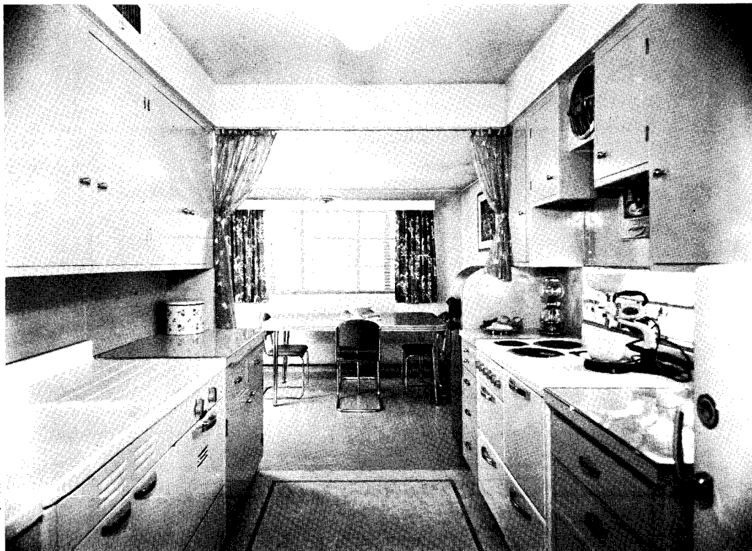
The kitchen is served by enclosed direct light and is equipped with electric range, refrigerator, water heater, combination sink and dishwasher, exhaust fan, food mixer, coffee makers, toaster, etc.
