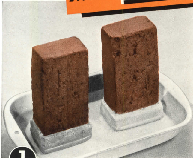
"Cap" one brick with Brixment mortar, and one brick with mortar made with portland cement and lime. After mortars have hardened, place both brick in a pan of shallow water. (Photo 1.) . . .
