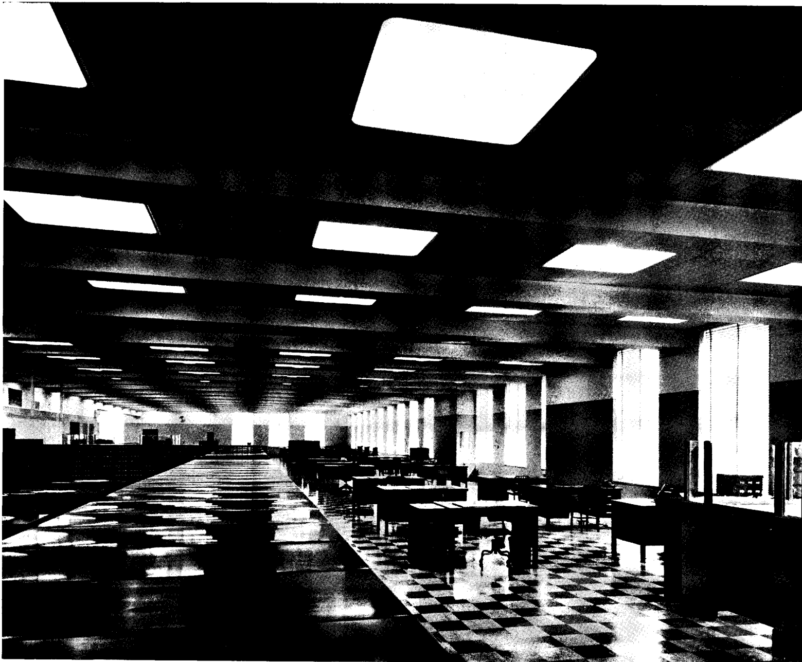
Typical workroom. Elimination of columns provides maximum flexibility for arranging desks or rows of file cases (at left).
