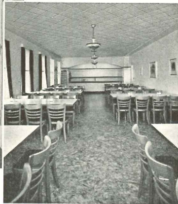
BELOW: Merritt Hospital, Oakland, California — nurses' dining-room. The 2000-sq.-ft. ceiling of Armstrong's Corkoustic, installed by Peterson-Cobby Co., San Francisco, keeps troublesome noise at a minimum. The material was specified by Ellard L. Slack, Hospital Superintendent.
