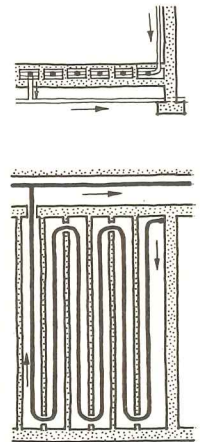
FIG. 23: Here air is heated in situ by pipe coils.
