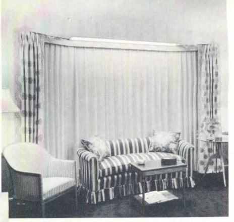
Illuminated soffit gives general illumination of room at night same general direction and distribution as in daytime
