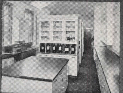
A BRIGHT, ATTRACTIVE pharmacy. Sink, table tops and counter tops are Monel.
