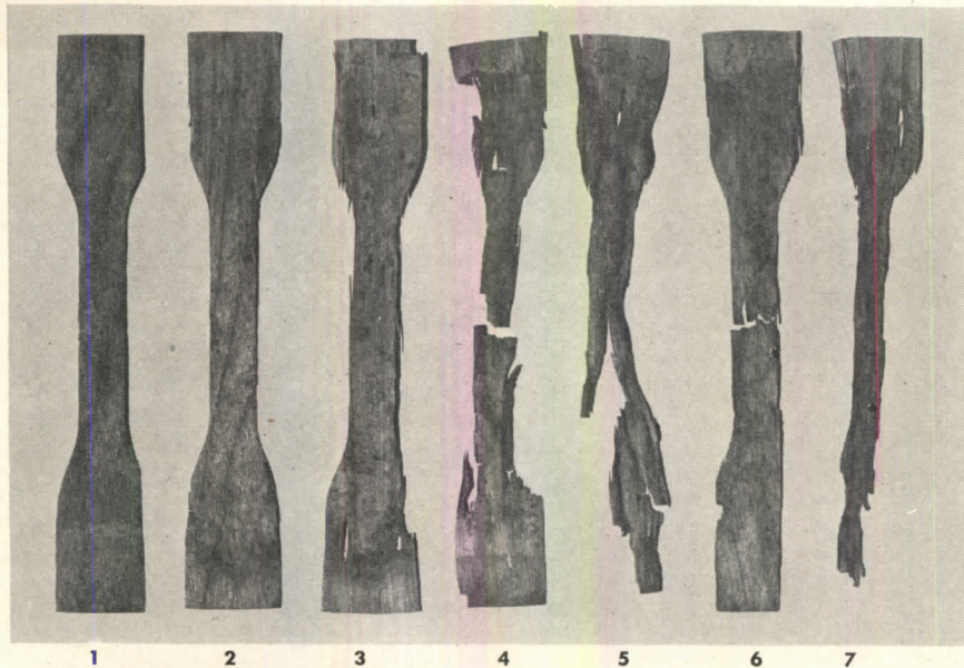
Result of 30 days' soil burial of yellow birch veneers dipped in the following preservatives: (1) Nuocide Copper (2 per cent); (2) Nuocide Zinc (4 per cent); (3) Nuocide Zinc (2 per cent); (4) and (5) other preservatives; (6) Nuocide Mercury; and (7) untreated
